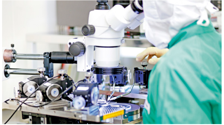
On-wafer chip characterization at Fraunhofer HHI
